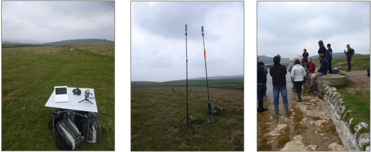
Figure 1. Enabling Remote Activity technology in use: an accessible base location (left) is connected to an inaccessible field site (right) using a portable wireless local area network (middle). A camcorder is used (right) to produce a live video stream and VoIP calls are used to provide a two-way audio link. Photographs taken on a WiFi camera can also be uploaded over the network to a web server at the base location.
